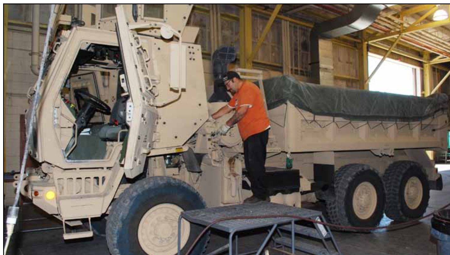
Rick Ramirez, heavy mobile equipment mechanic, uses a descaler to remove "carc" paint, making the area safe for welders. Carc paint is a type of paint used by the military on tanks which can produce toxic vapors when heated.
