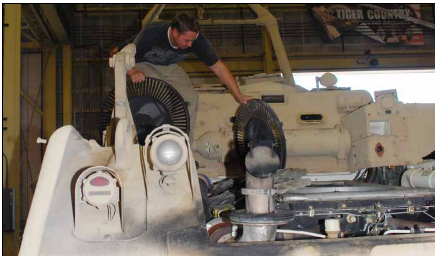
Brandon Ohm, heavy mobile equipment mechanic, removes engine fan covers to repair a fuel leak on an M88 Recovery Vehicle. (Photo by Mary Flores)
