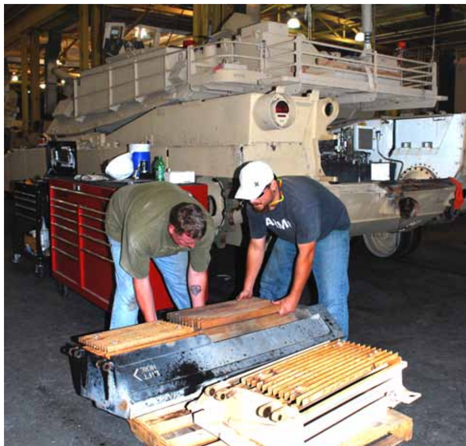
Ronald Beck (right) and Paul Wilson, both heavy mobile equipment mechanics, place the doors of an M1A1 Abrams on a wooden pallet to repair crack damages that occurred during testing.
