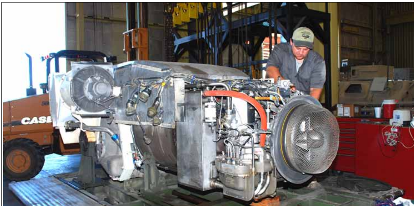
An auxiliary pump is removed for maintenance on an M1A1 Abrams Main Battle Tank engine by Anthony Pegram, heavy mobile equipment mechanic. (Photos by Mary Flores)
