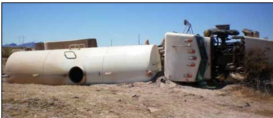
Water truck rests on its side after the truck’s front left tire blew out causing the truck to roll on the passengers side. The vehicle was totaled, however, fortunately, the driver was wearing his seat belt which prevented a worse outcome. (Loaned photo)
