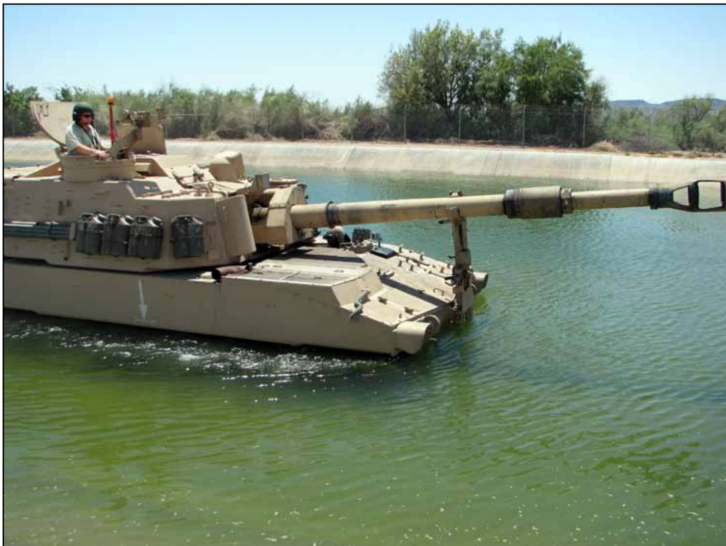
Soldiers need their self-propelled howitzers to be rugged and ready, no matter what. The M109A6 Paladin is expected to remain virtually watertight even when sitting in three-and-a-half feet of water for 15 minutes, a scenario that testers evaluate in YPG's fording basin. (Loaned photo)
