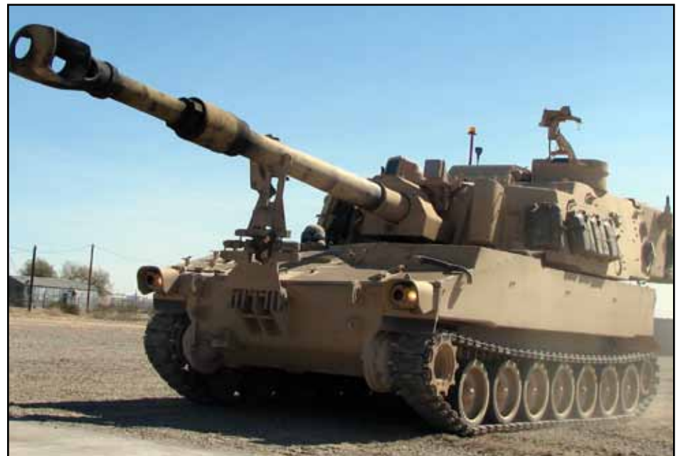
Firepower is only half of the story with the Paladin, and YPG testers subject the platform to more than 2,000 miles of rugged mobility testing during its stay. YPG's flexibility in testing complex platforms that require interdepartmental cooperation makes the proving ground stand out as a premier testing center. (Loaned photo)
