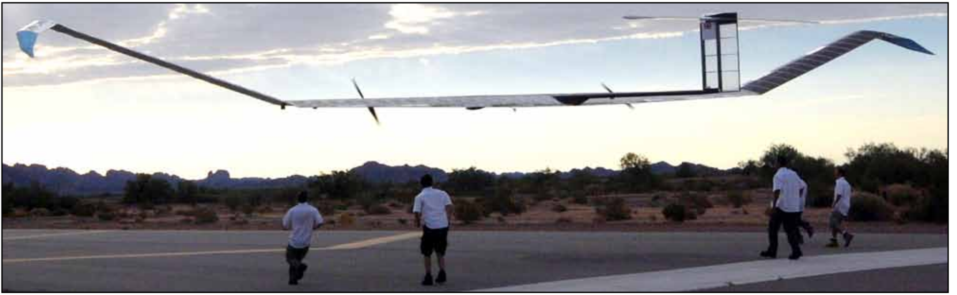
With a wingspan of 72 feet and weighing a mere 120 pounds, the Zephyr's two electric motors carry it as high as 70,000 feet above the ground. While the goal of this test is for the Zephyr to fly continuously for two weeks over Yuma Proving Ground, the ultimate objective is a craft capable of staying airborne for three months. (Photos by Mark Schauer)
