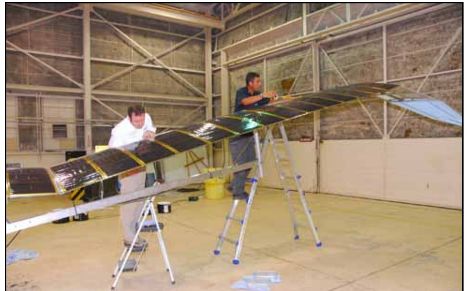
In the hours leading up to the Zephyr's launch, workers install protective coverings over the unmanned vehicle's solar-powered batteries. Hailing from England, the workers have tested different variations of the Zephyr at Yuma Proving Ground since 2008.
