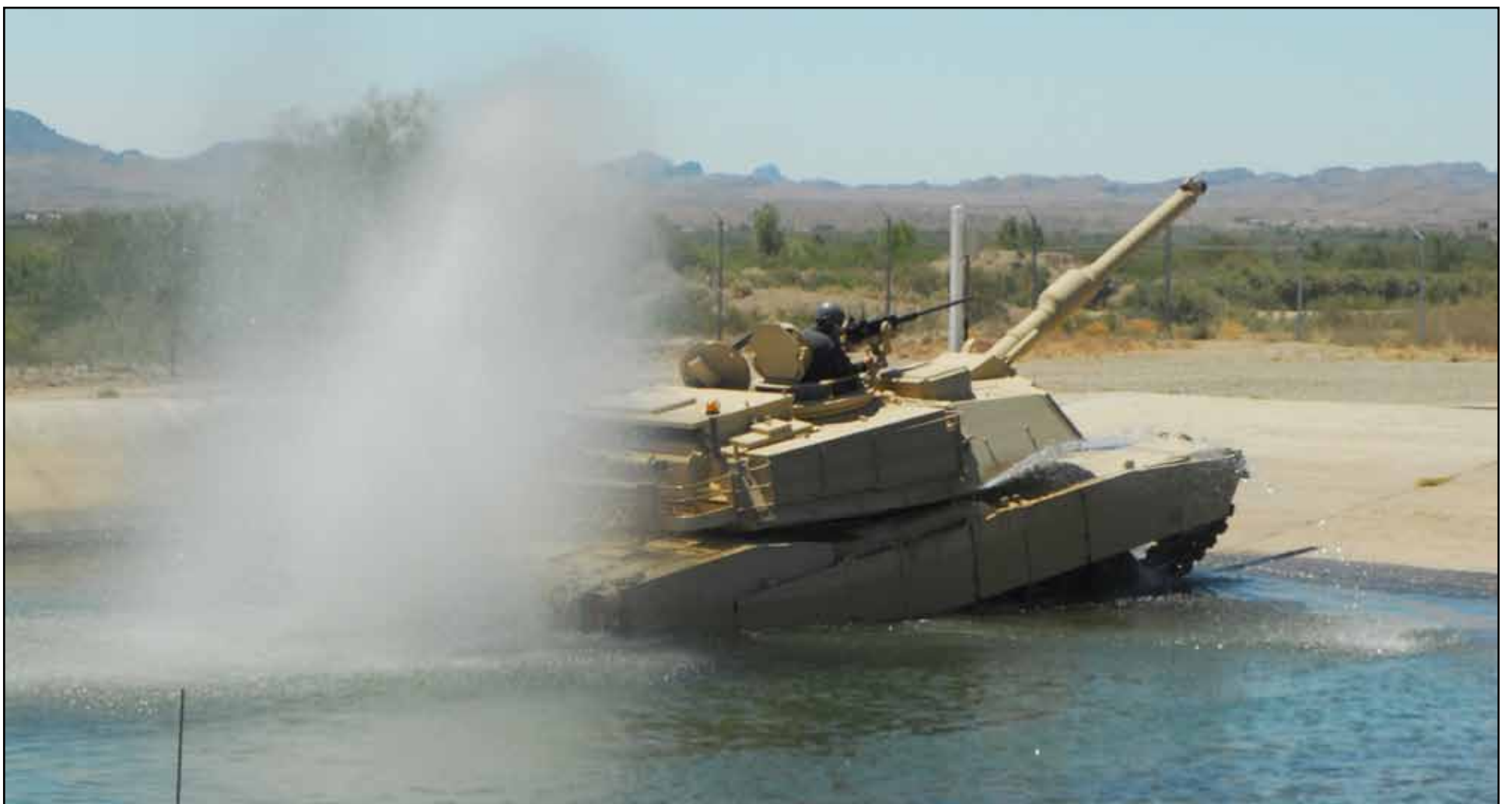
Water drips from an M1 Abrams as it roars out of YPG's fording basin. Filled with cold water from the Colorado River, the basin is frequently used throughout the year in the testing of armored vehicles. (Photo by Mark Schauer)
