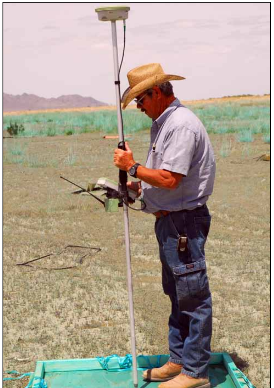
After the drop, geodetic surveyor Jerry Wells carefully measures and records where each of the 16 containers landed on the range. The blue dye that marks where the water landed fades after several hours in the sun, long after a recovery crew has gathered up the remains of the PCADS' cardboard sleeves and plastic blivets.
