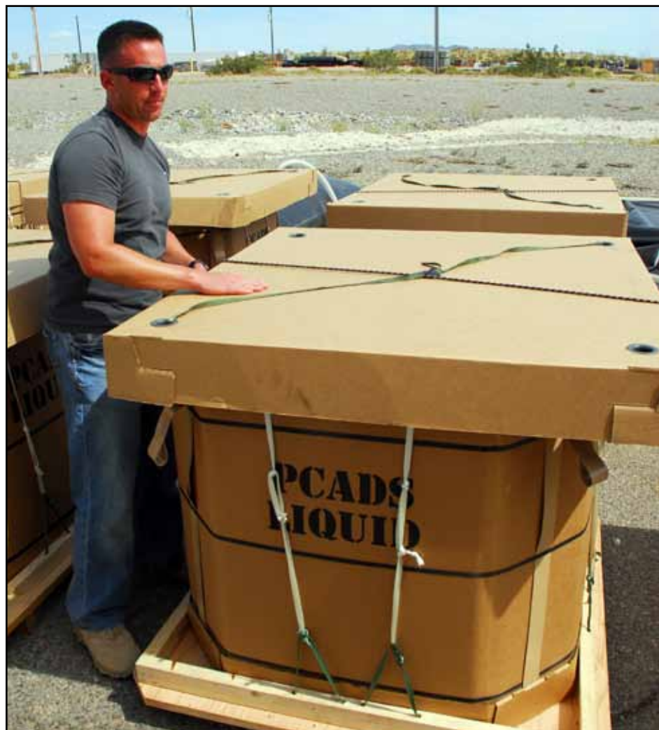
YPG test officer Keith Allen adjusts the nylon cord on the tri-wall cardboard sleeve that gives the water-filled polyurethane bag shape. Once rigged, the containers can be loaded like any other air cargo, which makes fighting forest fires easier for Air National Guard crews.
