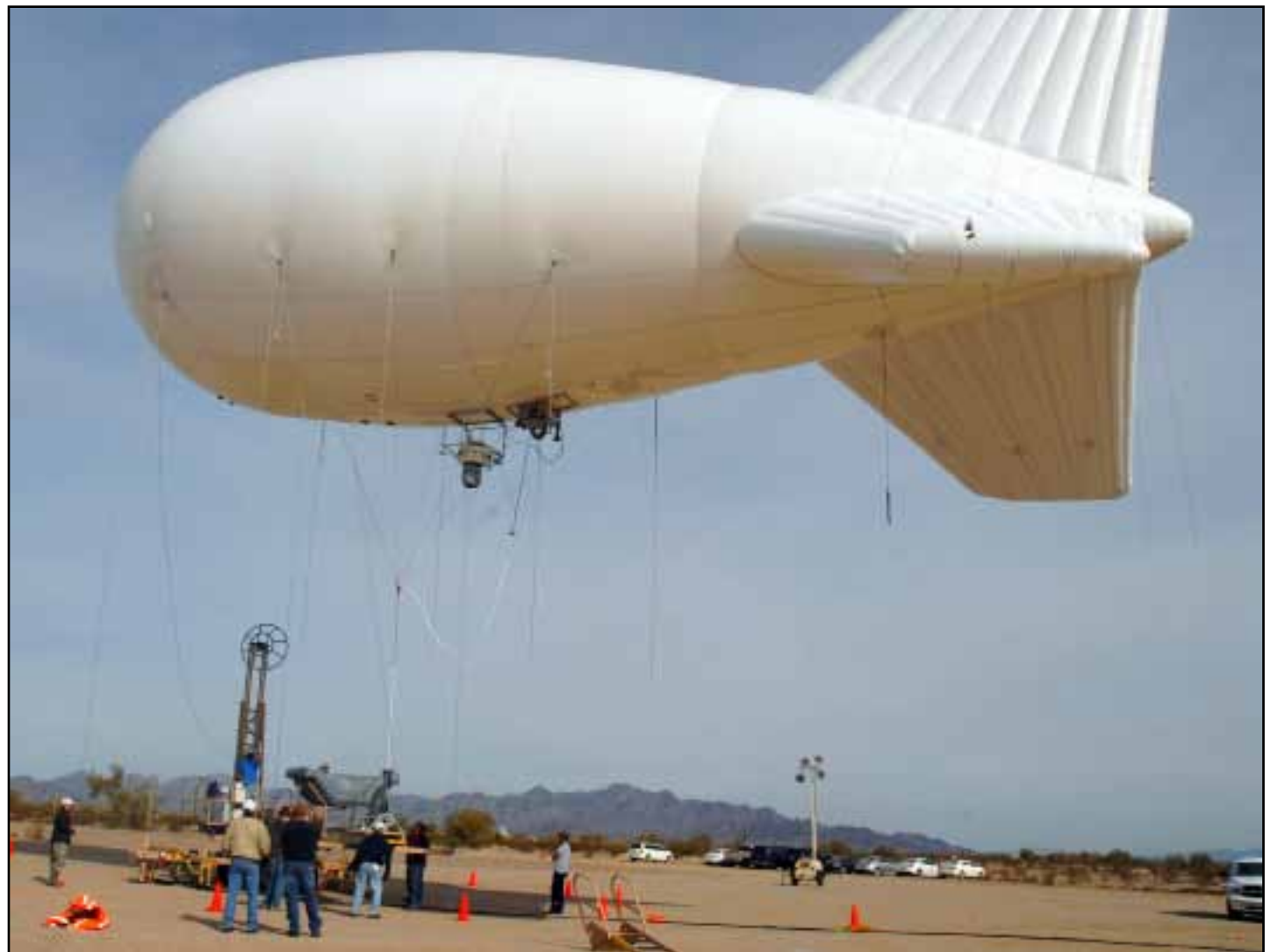
Persistent Ground Surveillance Systems (PGSS) marry cutting edge high-tech detection sensors to an ordinary blimp. The moored lighter-than-air craft can float as high as 3000 feet above the ground, lofting a sensor suite that allows ground controllers to continuously monitor a huge swath of land. "As soon as they're done at YPG, they'll be deployed to various points around the world," said Shawn Greene, the NACCITEC test officer in charge of the evaluation.
