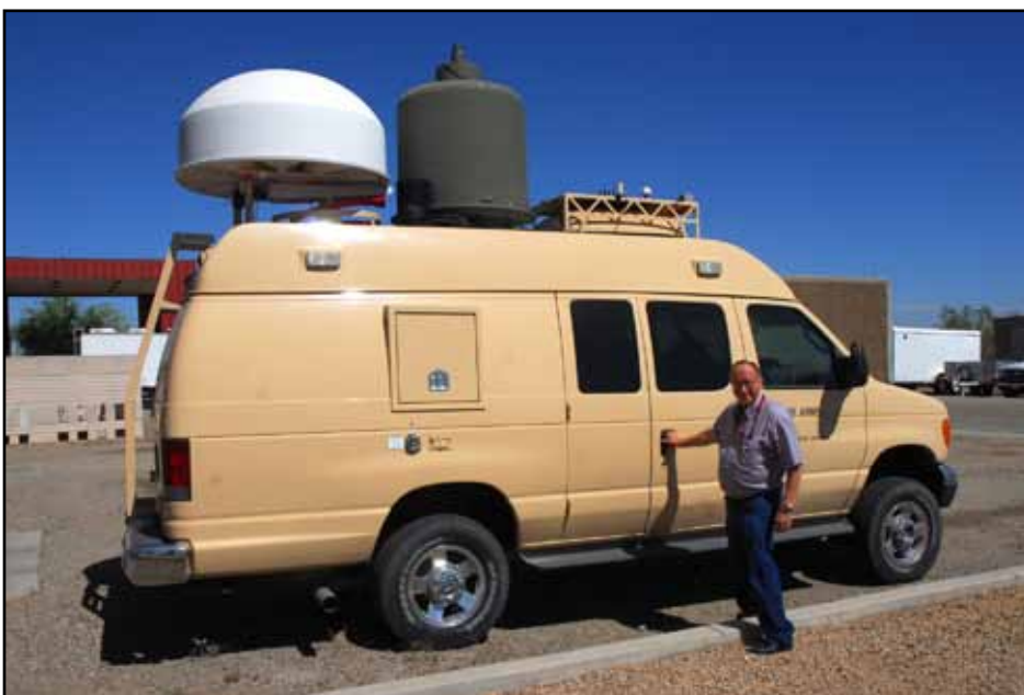
A new radio van is among the recent equipment upgrades that benefits the spectrum management office. The mobile station is outfitted with two direction finding radio antennas and a bevy of computers for operation of YPG's spectrum monitoring network.
