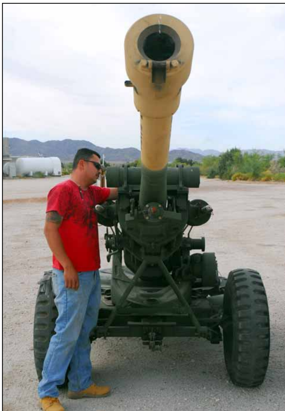
Weapons maintenance mechanic Jose Roque inspects a recently fired M119 howitzer. YPG evaluators pay particular attention to the weapon's recoil during test fires: a recoil that is not to specification can quickly cause other problems in the system, which could prove fatal to troops in the field.
