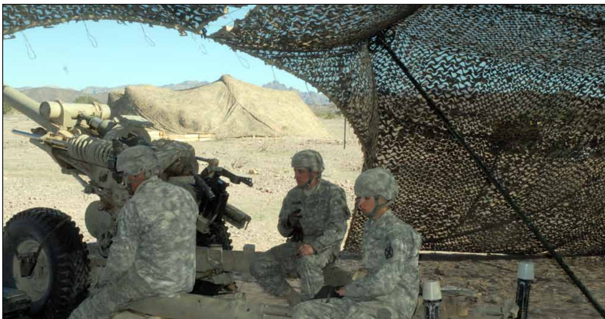
Though not the biggest howitzer in the Army inventory, Soldiers like these undergoing training at YPG from Fort Drum, N.Y., find the M119's portability useful. The weapon is light enough to be parachuted into inhospitable mountain terrain found in places like Afghanistan, and can be easily and rapidly emplaced for use. (Photos by Mark Schauer)
