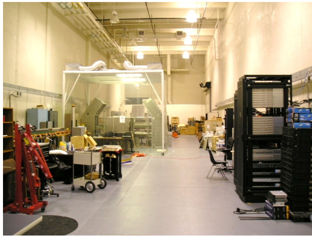
Figure 18: Florida Tech high-bay experimental area with 200 ft 2 clean room (class 100).
