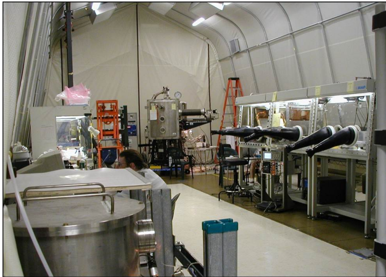
Figure 20: The Stony Brook University clean room featuring a class 100 tent, class 1 laminar flow table, high vacuum evaporator, and large volume glove box.
