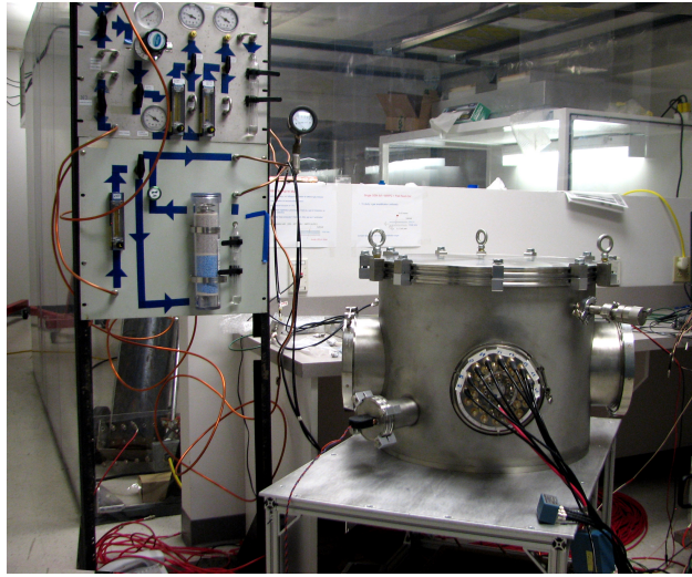
Figure 24: Yale GEM R&D laboratory showing the general purpose test vessel, gas system and (in the background) clean area with laminar flow bench.
