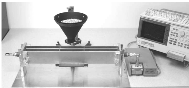
Figure 1. Master transmission-line test cell, loading funnel and HP-4291A RF Material/Impedance Analyser.
