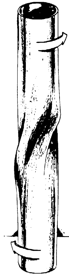
Figure D-6. Torsion load failure
