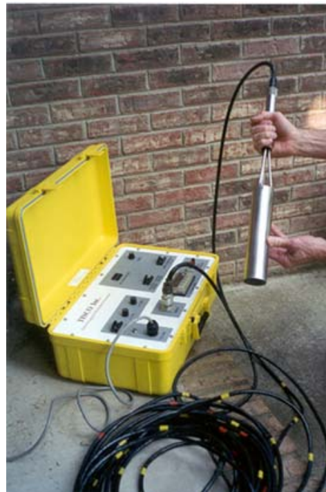
Figure 4-1. Electromagnetic borehole flowmeter (EBF) ( www.qec-ebf.com ).
