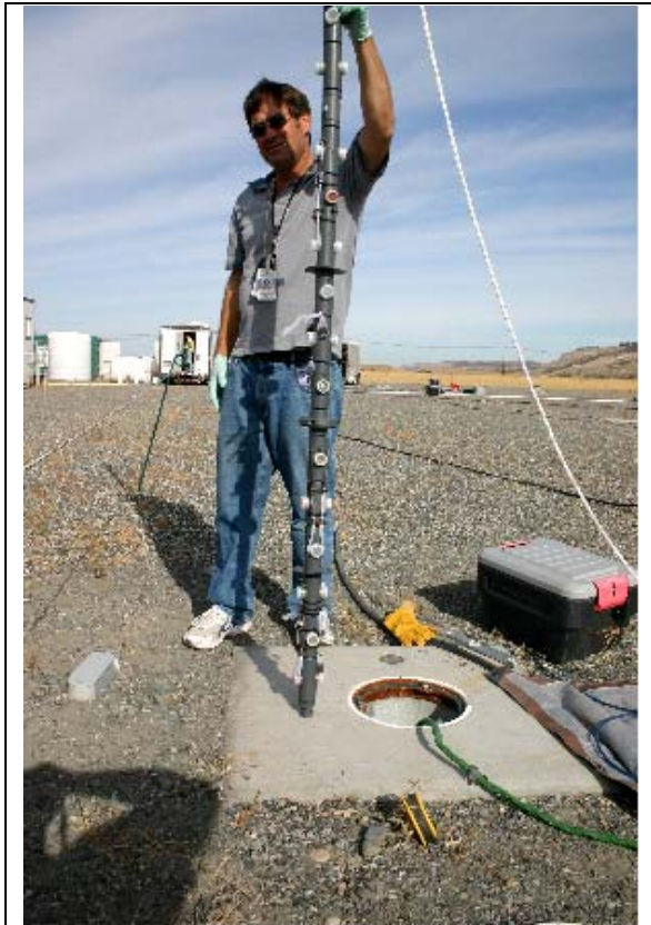
Figure 10. One of three microcosm strings deployed to well 3-24 by PNNL SFA researchers for in-situ biogeochemistry studies.
