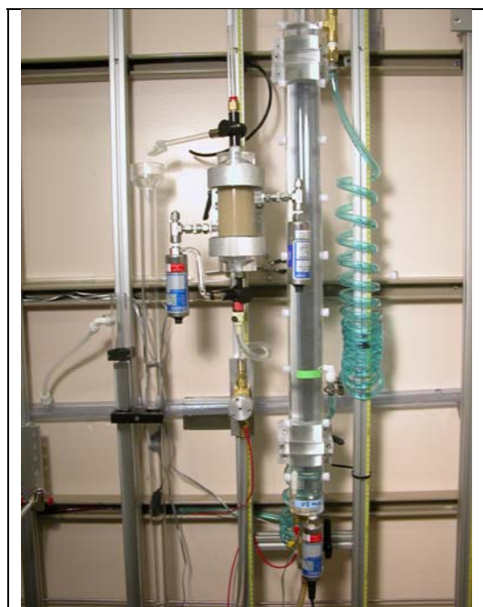
Figure 5-8. Apparatus for automated, laboratory measurement of sediment hydraulic properties (k-S-p relations) in EMSL (SFTEL).
