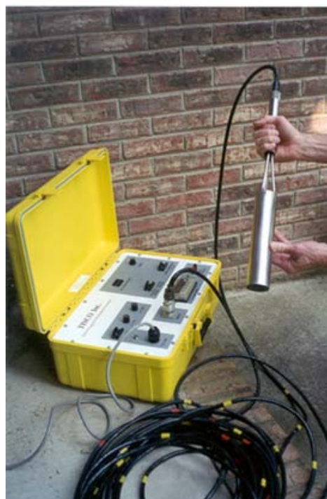
Figure 4-1. Electromagnetic borehole flowmeter (EBF) ( www.qec-ebf.com ).
