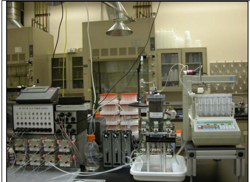
Figure 4. Experimental apparatus for intact core experiments including perfusion pumps, synthetic groundwater reservoir, 4” intact core with pressure transducers, and fraction collector for effluent sampling.
