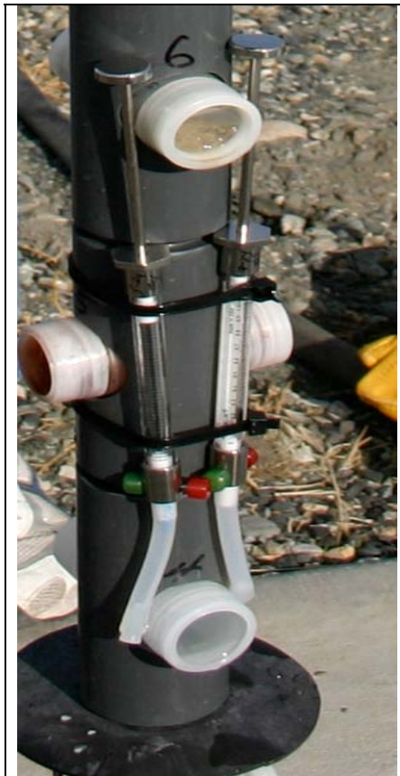
Figure IV-6. Passive multi-level sampler showing cells containing solids for microbiological experiments and water for aqueous geochemical analyses. Dissolved gas samplers (air-filled gas syringes) shown in photo on left were shipped to ORNL (B. Spalding and S. Brooks) for analyses immediately upon removal of the MLS.
