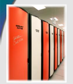
Jaguar: 11,508 dual-core 2.6GHz AMD Opteron processors, 4 GB of memory (2 GB per core) for a total of 46 TB, 600 TB of scratch space, Cray Seastar router through Hypertransport interconnected in a 3D-torus topology providing very high bandwidth, low latency, and extreme scalability.
