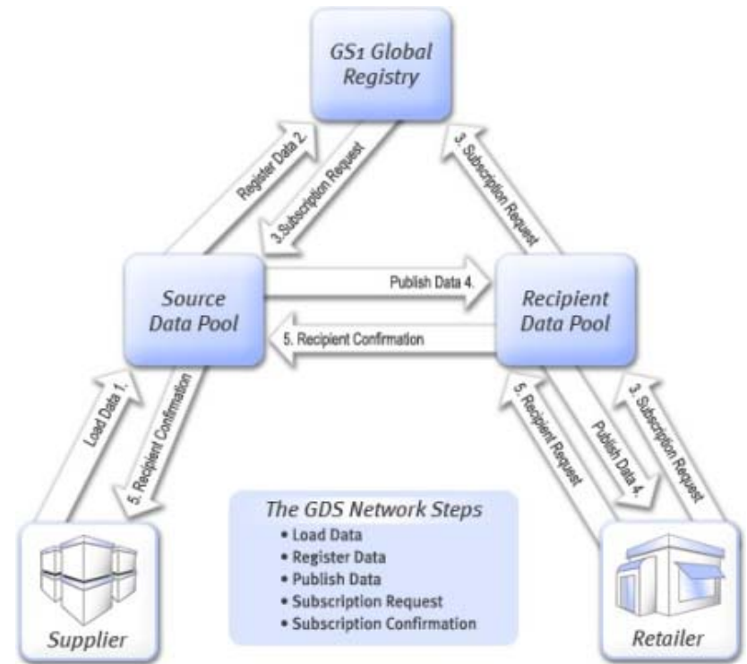
FIGURE 3: Data flow in the Global Data Synchronization Network. ACE would function as another Retailer that consumes product information published by Suppliers.
