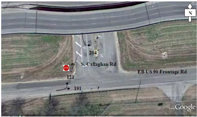
Figure 3.1. AM Peak Hour - East Bound US 90 Frontage Road at S. Callaghan Road
