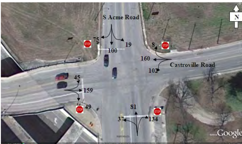
Figure 3.4. AM Peak Hour - Castroville Road at S Acme Road
