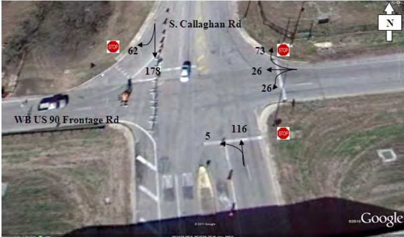
Figure 3.2. AM Peak Hour - West Bound US 90 Frontage Road at S. Callaghan Road
