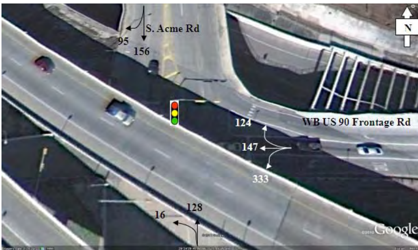
Figure 3.6. AM Peak Hour - S. Acme Road at West Bound US 90 Frontage Road
