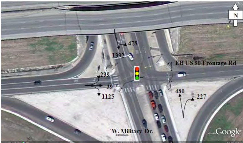
Figure 3.9. AM Peak Hour - W. Military Drive at East Bound US 90 Frontage Road
