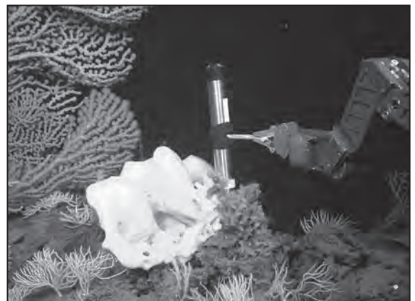
Current meter placed near corals and sponges at the top of Davidson Seamount to measure local currents
