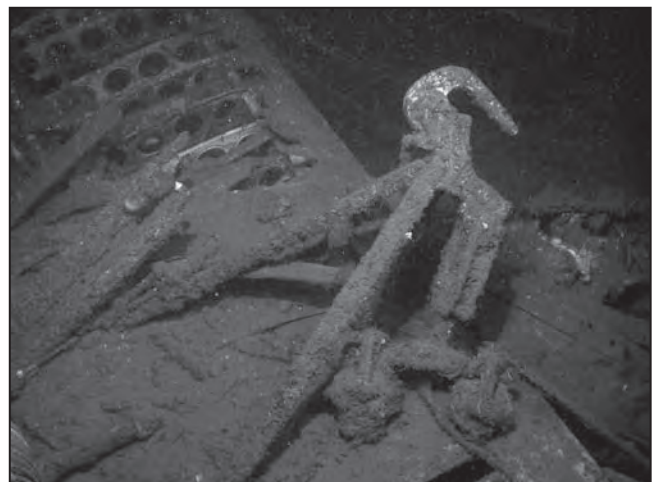
Submerged view of the sky-hook located at the center of the Curtiss Sparrowhawk F9C-2 biplane. During flight, the pilot positioned the aircraft below the Macon's hangar, where a trapeze was lowered; the pilot positioned the hook onto the trapeze. Sparrowhawk pilots were nicknamed the 'men on the flying trapeze.'
