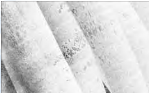
Figure 2. Side scan sonar mosaic of a sandy bottom area, 105 by 162 meters, off Pacific Grove, showing squid egg mops in the central region.
