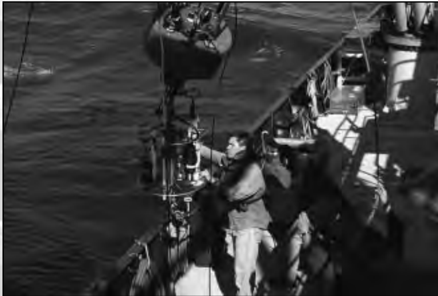
MBARI scientists deploy an OASIS drifter from the R/V New Horizon, a Scripps Institution of Oceanography vessel.
