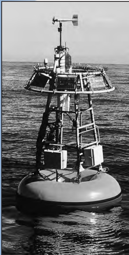
Moorings gathered at sea are equipped with sensors that gather data on water chemistry, meteorological conditions, currents, and temperature.
