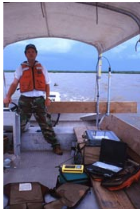
Figure 2. USGS scientists logged simultaneous depth measurements and GPS positions across the lakebed at high water every 6-10 feet (2-3 m) along transects spaced at 0.6-mile (1-km) intervals.
