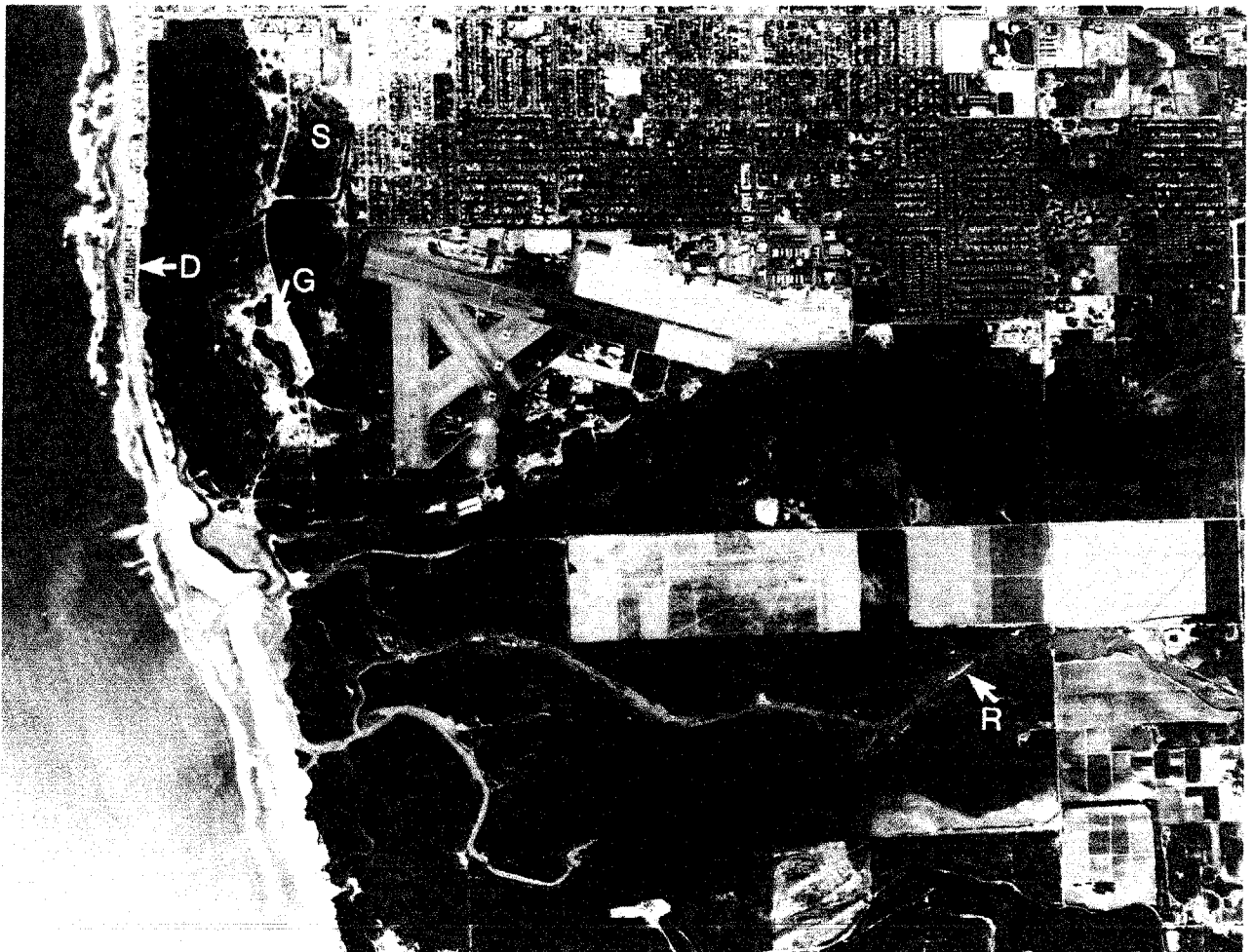
Figure 11. The February 18, 1978, aerial photograph of Tijuana Estuary (from Aerial Fotobank). Note development on beach (D), abandoned sewage oxidation ponds (S), gravel excavation (G), agriculture (A), and location of main river channel (R).
