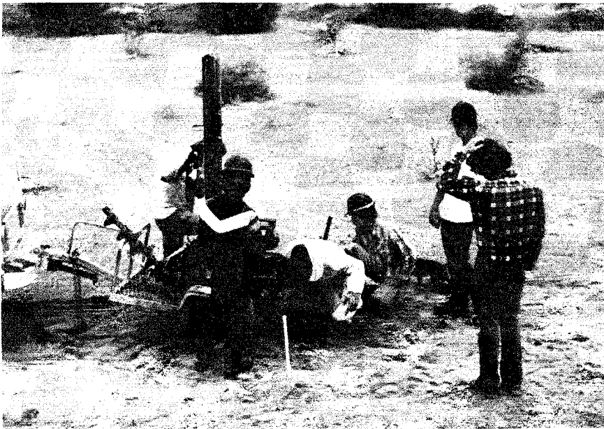
Figure 38. Augering holes to the water table and collecting soil, water, and salinity data are all essential steps in determining the growth potential of native riparian trees and shrubs. Photo by J. Disano.
