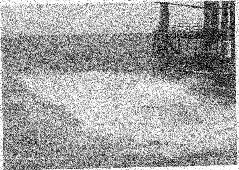
Mud discharge contacting surface near platform.
