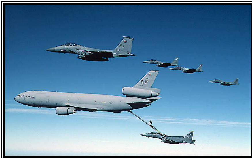
Figure 8. A KC-10 Extender conducts refueling operations for an F-15 Eagle (U. S. Air Force)
