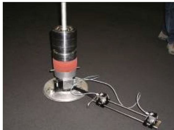
Figure 11: Lightweight Deflectometer (LWD)
