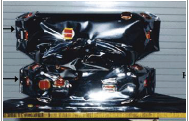
Figure 1. Pre-launched TiPS end-masses. Spring-powered mechanism separates the end-masses at tether deployment. The masses were affectionately dubbed Ralph and Norton for the two principal characters in the classic TV series "The Honeymooners" (courtesy, Dr. Shannon Coffey, NRL).
