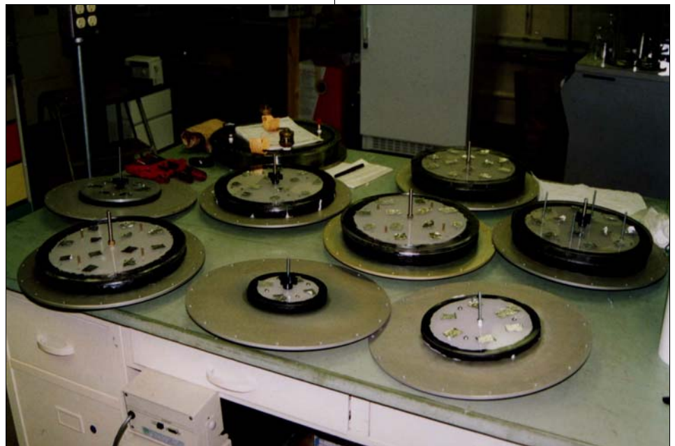
A few of many simulated puncture sample plates, with patches installed, produced for ground testing. These were injected with adhesive in normal gravity and tested for seal effectiveness at one atmosphere. Patch thickness and diameter vary, depending on hole size and module wall irregularities.
