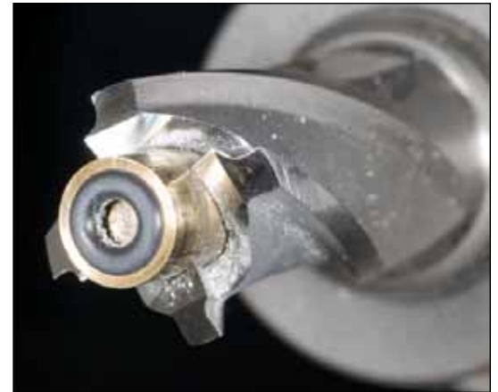
Figure 1. The coring device developed at JSC, shown immediately after a coring test. Cores taken have a diameter (measured at the core's painted surface) of approximately 7 mm, corresponding to the inner diameter of the annular cutter. Minor paint flake abrasions are seen inside the cutter; other debris are contained within the vacuum shroud (shown in Figure 4). The device is cleaned and inspected after each operation.
