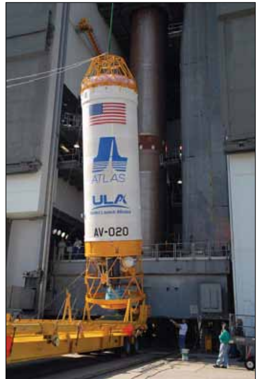
Large launch vehicle orbital stages, like this Atlas V Centaur stage, can pose human casualty risks exceeding widely accepted norms.
