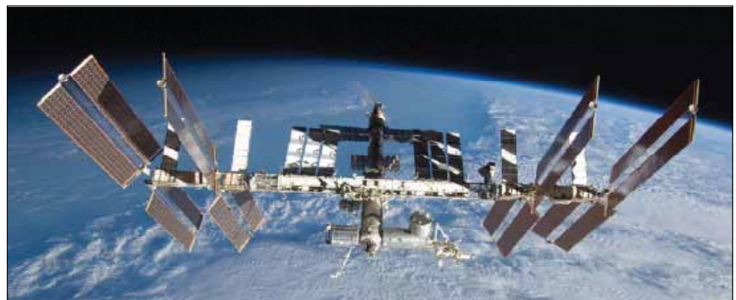
With a breadth of more than 100 meters, the International Station Space presents a large target for orbital debris.
