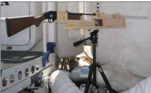
Figure 3. The air gun supported in its tripod-mounted cradle. The red-edged box in the forward part of the cradle is the ballistic chronometer.
