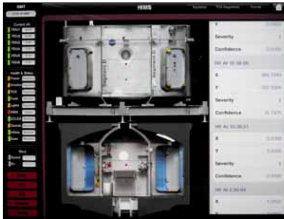
Figure 2. The HDU Crew Display iPad, showing the HIMS alert screen. Impact locations are highlighted on the images while numerical results appear in a scrolling table.
