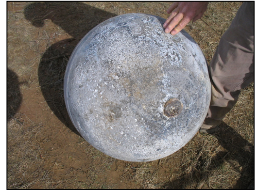
Pressurant tank found in Colorado in March 2011 and tentatively linked to a Zenit launch vehicle stage.
