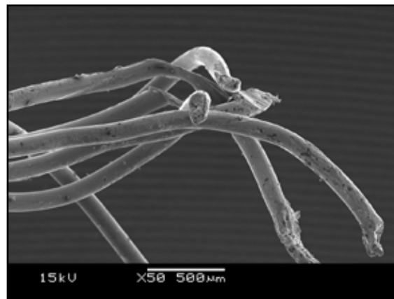
Figure 2. Frayed end of 4B SAW guidewire. Wires at bottom and in lower right-hand corner exhibited melt near ends.
