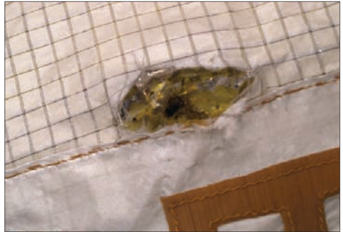
Figure 1. Damage to FGB thermal blanket observed by RS EVA-19 crew. Note, each square on the exterior fabric of the thermal blanket is \sim 1 cm x 1 cm. The tear in the exterior fabric cover is 6.7 cm x 3.3 cm and the hole in the underlying thermal blanket layers is 1.0 cm x 0.85 cm.
