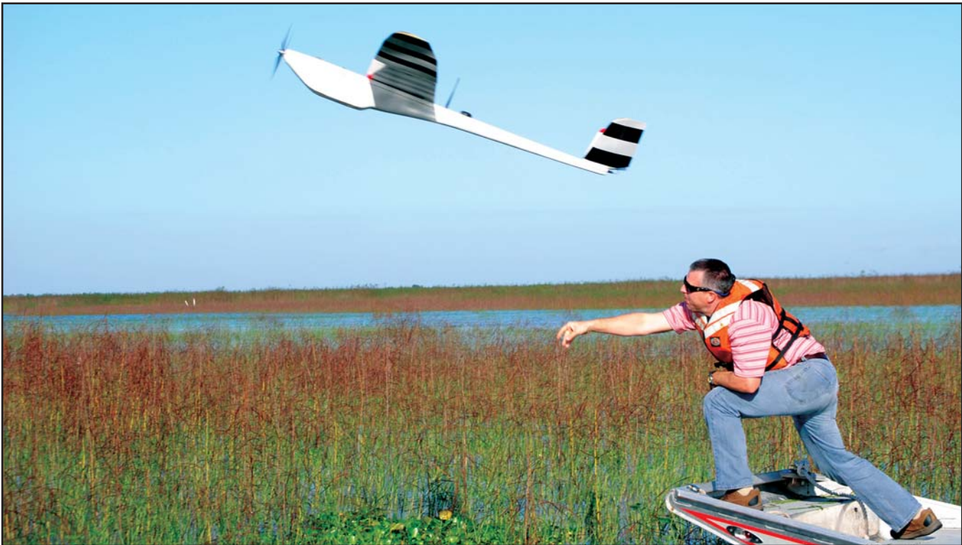
With a mighty heave, Damon Wolfe, a geodesist with the Jacksonville District, launches the NOVA UAV on a flight over Lake Okeechobee. The Corps used photos from the UAV to track the progress of various plant species at the lake.
