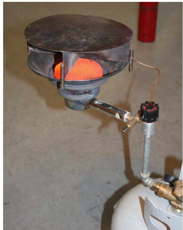
Propane heater used to conduct "pop tests" at the PMC seed cleaning facilities.
