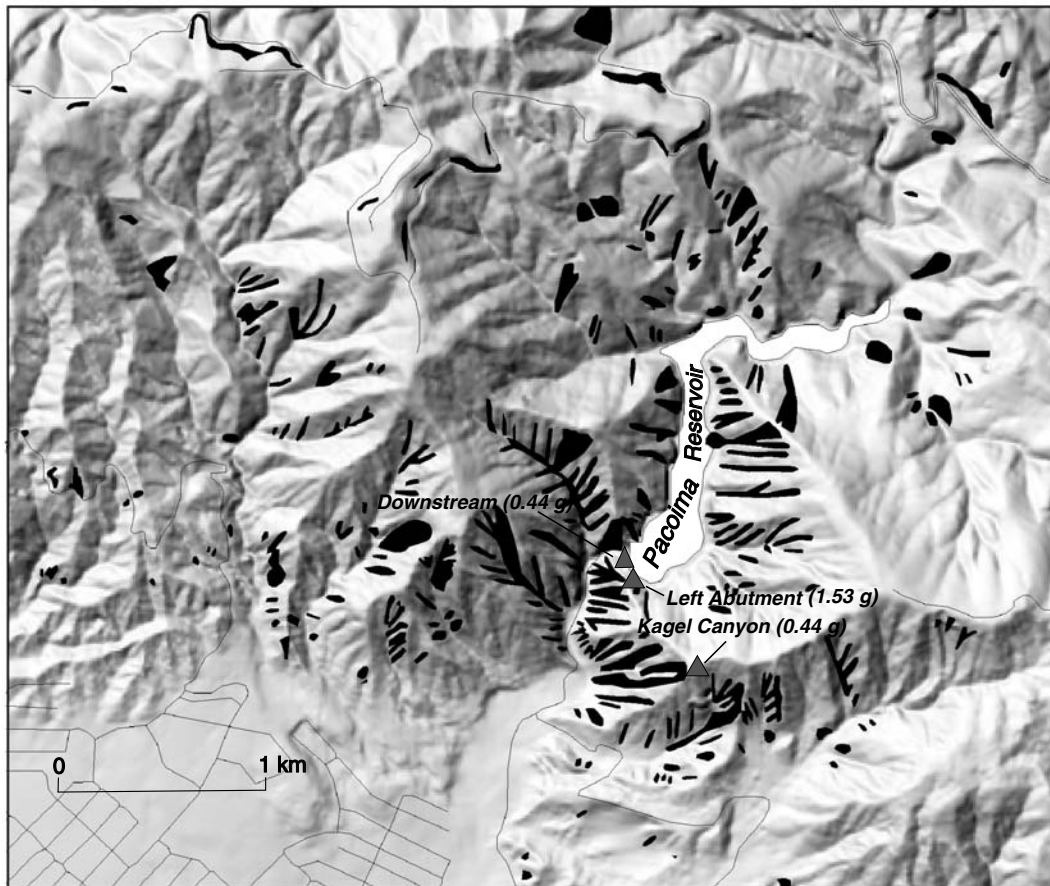
Figure 6. Landslides triggered in 1994 in the vicinity of Pacoima Canyon along with the locations of three strong-motion stations and their respective peak accelerations. Note that landslide concentrations occur on both sides of the ridges defining Pacoima Canyon. Location shown in Figure 2.
