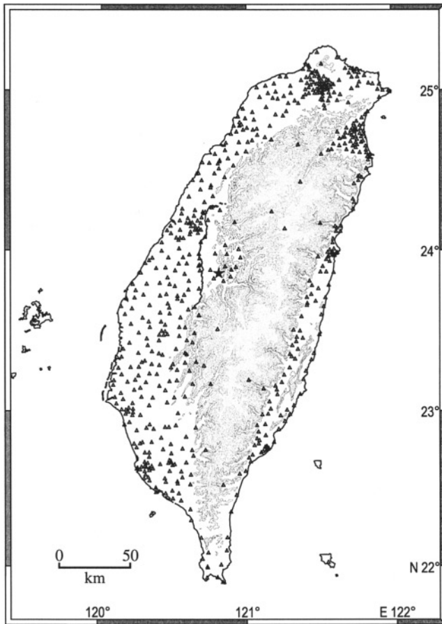
Figure 1. Locations of the free-field, three-component, digital accelerometer stations. The star indicates the location of the mainshock. Surface ruptures extending about 80 km in a nearly north-south direction are shown by the jagged line to the left of the mainshock (from Lee et al. , 1999).
