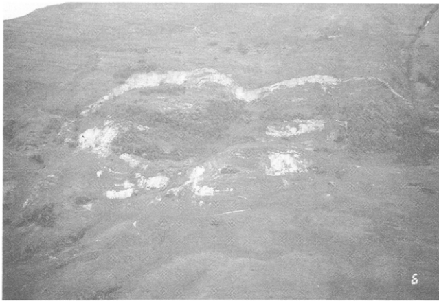
Figure 13. Rock block slide on slopes above Shkmeri. Landslide block rotated counterclockwise. Scarp on left side of photo has about 50 m of displacement.
