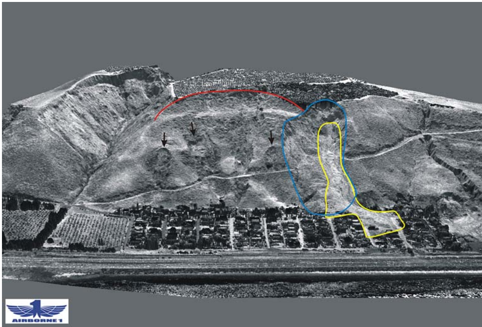
Fig. 4 Oblique LIDAR image of La Conchita after the 2005 landslide. Outline of 1995 (blue) and 2005 (yellow) landslides shown; arrows show examples of other landslides in the area; red line outlines main scarp of an ancient landslide that involved the entire bluff. The deep canyon
