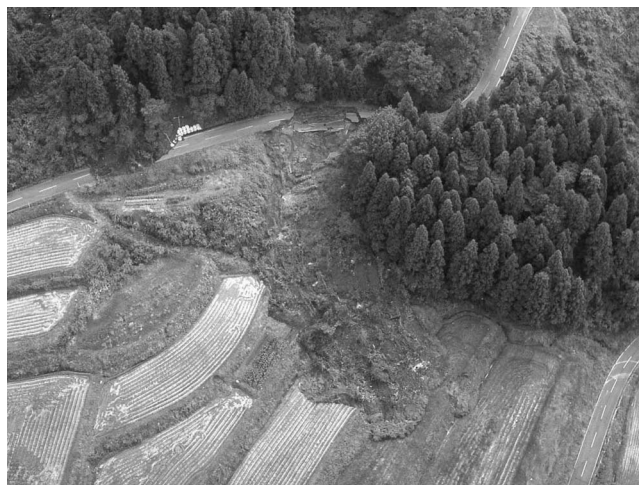
Figure 17. Slump-flow complex in a colluvium-filled swale along Highway 9 east of Nagaoka (photo: I. Yasuda, Hasshu Company).
