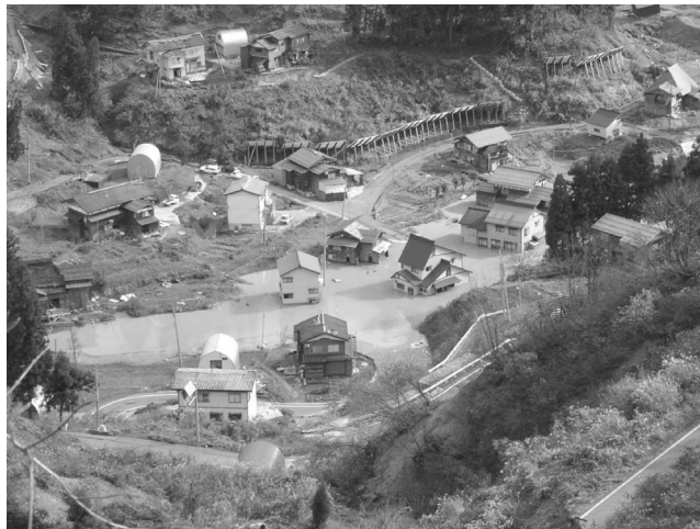
Figure 22. Looking east from Road 23 at the inundation of a tributary valley and houses upstream of a landslide dam in the Yamakoshi epicentral area.
