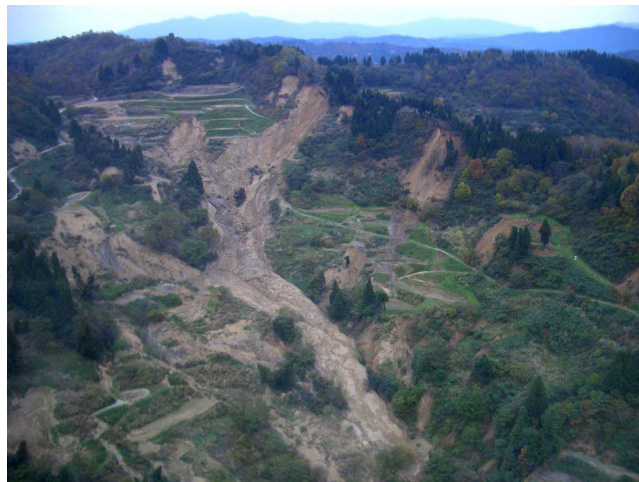
Figure 20. Large debris flow, exhibiting a narrow path and a long runout.
