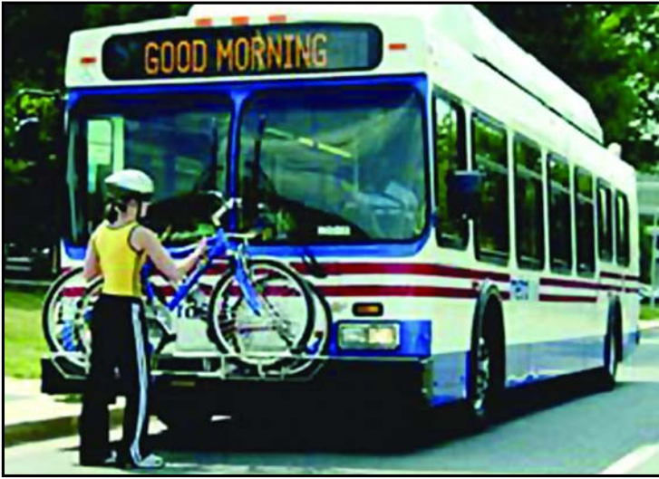
Metrobuses operating in the District of Columbia are equipped with bicycle racks.
