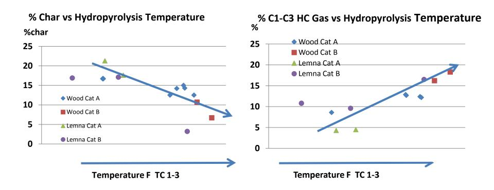
As Hydropyrolysis temperature goes up, Char goes down, Gas goes up
