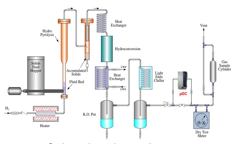
Continuous char-catalyst separation, Improved light gasoline recovery
