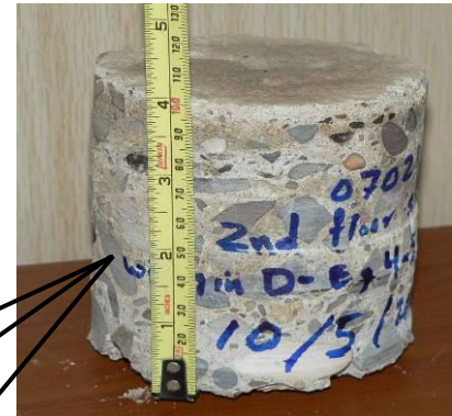
Site Photo 7. Evidence of low concrete strength (Courtesy of the USACE)
