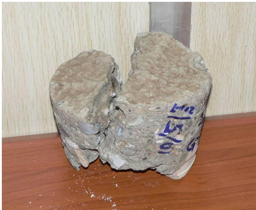
Site Photo 5. Concrete core sample that cracked, indicating extremely low strength (Courtesy of the USACE)
