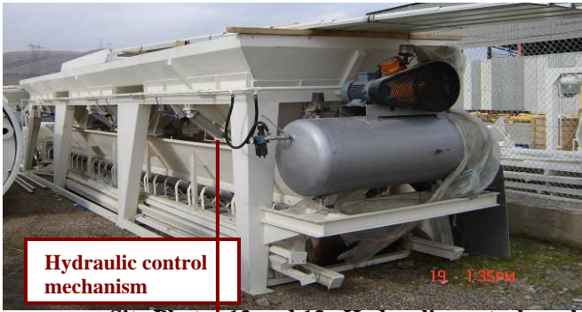
Site Photos 12 and 13. Hydraulic control mechanism and aggregate handling components with for the delivered 30-m 3 /hour concrete-mixing plant.
