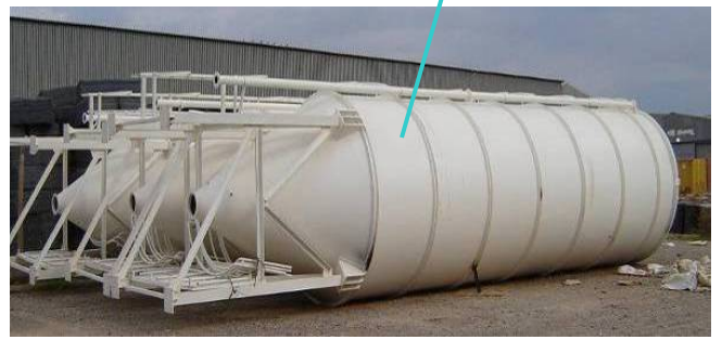
Site Photo 15. Three silos (two needed for each mixing plant)
