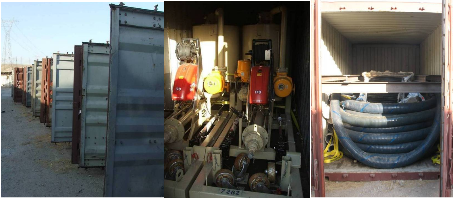
Site Photos 30, 31, and 32. Conex boxes with partially assembled enhanced grouting equipment
