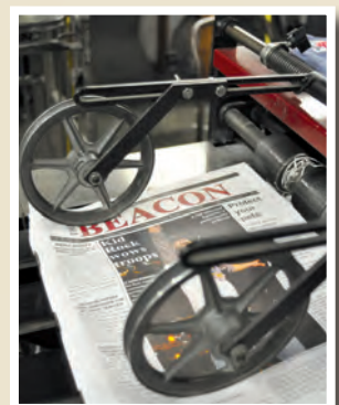
So much for "hot off the press!" The Beacon actually comes out cold and wet off the press due to the use of water in the printing process.
