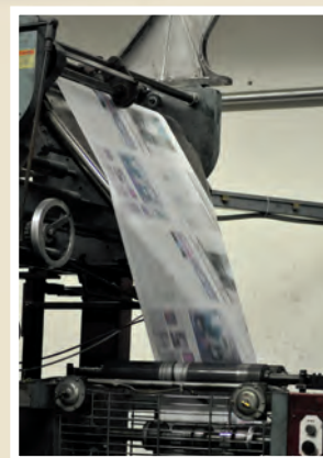
Once the machines are calibrated, the final product prints on a jumbo roll of paper. More machines fold and cut The Beacon into its familiar shape.
