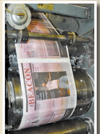
Technicians place the plate, ink and other materials into the giant printing press and print test copies.
