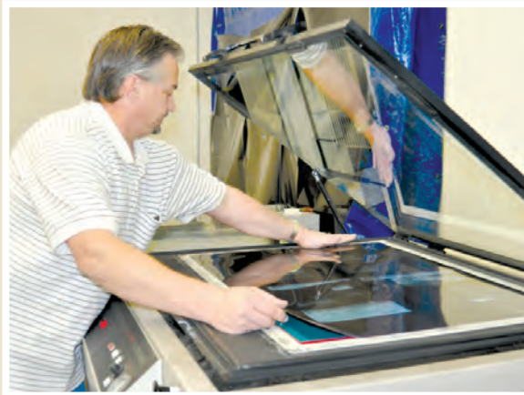
The editor sends the digital copy to Aerotech News and Review. The staff create a negative film and a three-foot metal plate for printing.
