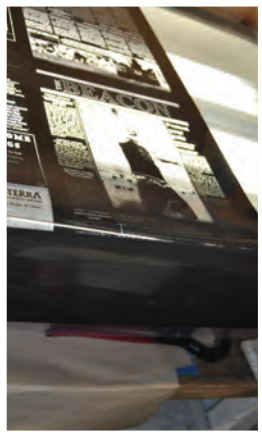
The editor sends the digital copy to Aerotech News and Review. The staff create a negative film and a three-foot metal plate for printing.
