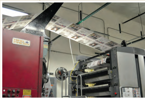
Once the machines are calibrated, the final product prints on a jumbo roll of paper. More machines fold and cut The Beacon into its familiar shape.
