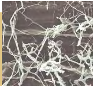
Brown-rot fungus, Postia placenta , breaks down hemicellulose and cellulose (Forest Products Laboratory)
